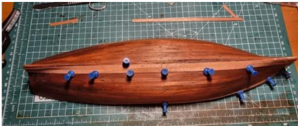
Photo left shows one technique of securing planking during gluing.
