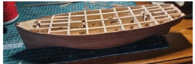
Photo above shows the completed planked hull and fore and aft bracing. This model's laser cut tolerances were quite loose, so bracing was required to keep all the rib sections true and square.
