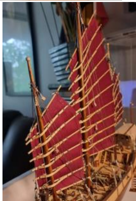
Above centre Sails in place with the secondary batons ends secure towards the leech end of the main batons
