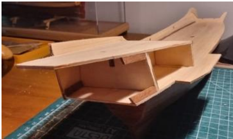
Photo above shows the completed planked hull and fore and aft bracing. This model's laser cut tolerances were quite loose, so bracing was required to keep all the rib sections true and square.
