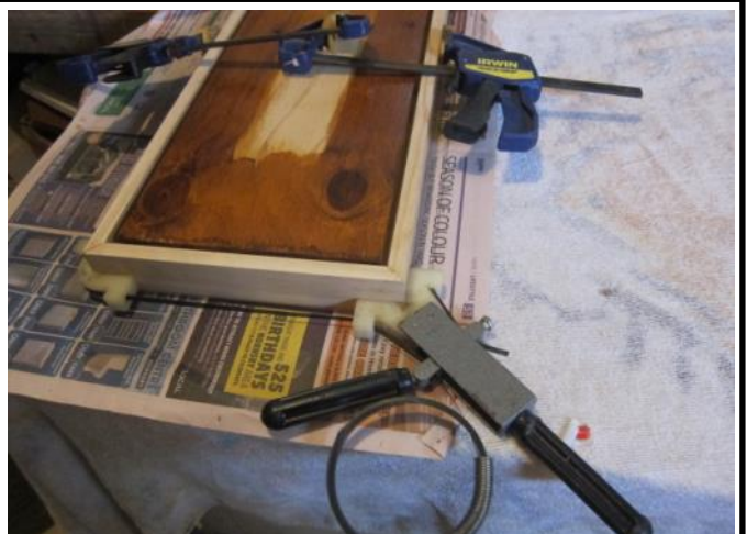
20. A view showing the mitre clamp and two clamps. There are many other styles of mitre clamps.
