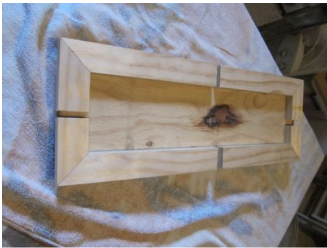
15. All timber pieces glued to base.
