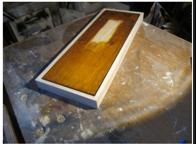
22. The clamping is removed and the cover strips have been sanded ready for staining.
