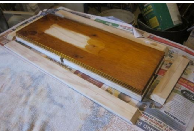
19. The four cover strips have been cut to length and mitred. Much care is required when producing these pieces. The job now rests on newspaper before gluing.
